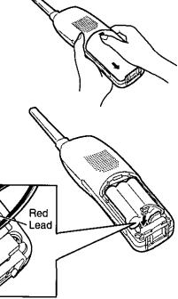
Close the cover. Be sure to charge the new battery for about 15 hours.
